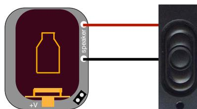
Note that you **must** disconnect the internal loudspeaker before connecting an external one otherwise you will overload the amplifier circuitry. NB The SFX speaker is bonded to the main microchip - not recommended to try & remove!
