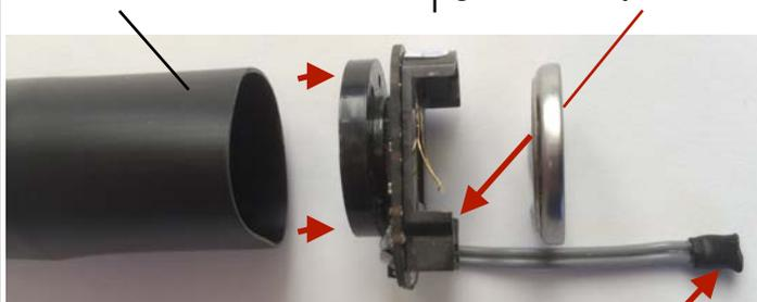
This is the Motion Sensor - always locate this **away** from speaker and not touching other surfaces in the model as it is very sensitive!
