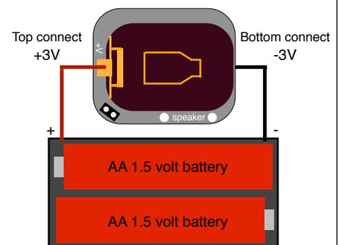
**WARNING:** Correct polarity & 3 volts MAXIMUM!
